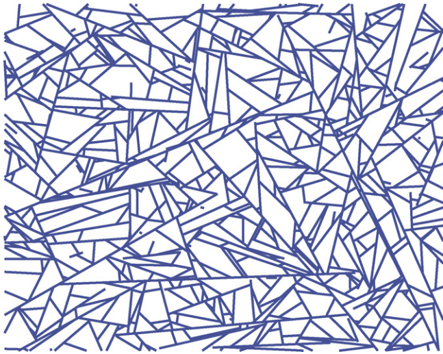
Fig. 4. Simulation of one layer of carbon fiber in a GDL.
